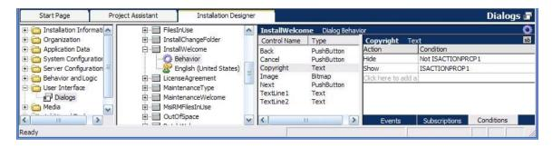
At run time, if a previous version of the product is not detected, the modified text control will be hidden:
